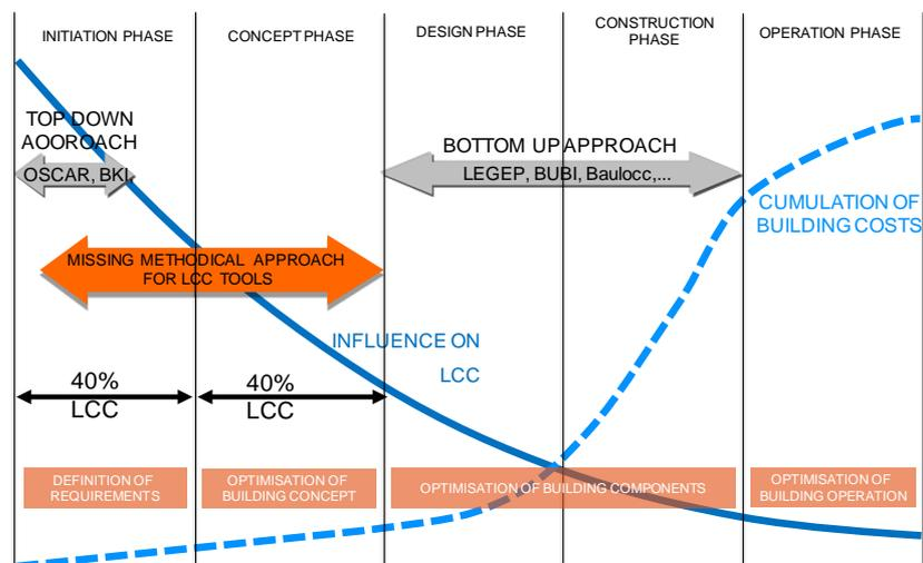
Figure 1: Missing link in models for calculating life cycle costs during the design phase (Source: original illustration)
